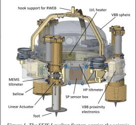
Figure 1. The SEIS Leveling System carries the seismic sensors
