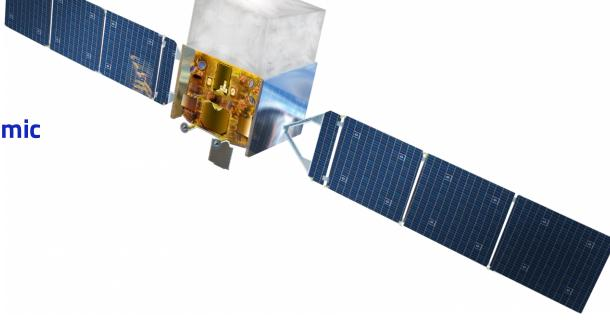
The ACD consists of an array of plastic scintillator tiles, which emit light when traversed by charged particles. By detecting these particles, the ACD helps identify and reject events caused by charged particles, allowing the LAT to focus on gamma-ray signals.
