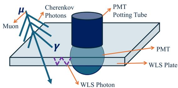
Figure 1 – Schematic of PMT embedded in the center of a WLS plate, demonstrating the light guiding affects.
