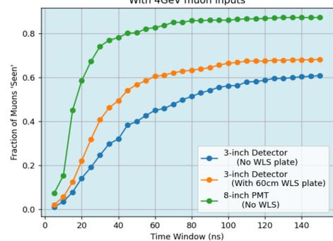
Figure 6 – Fraction of muons detected using a 50-photon threshold, for a 3-inch PMT with and without WLS plates and an 8-inch PMT.
