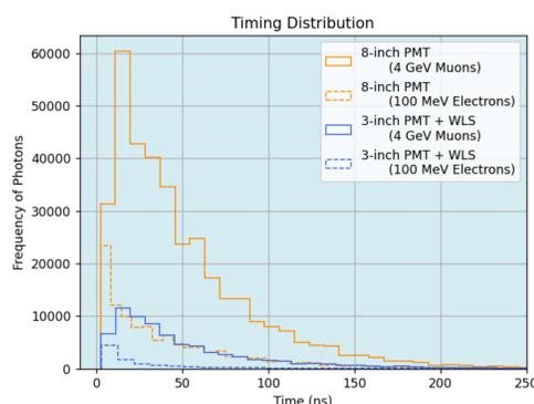
Figure 5 – Timing distribution between electrons and muons for a 3-inch PMT with WLS plates and an 8-inch PMT.
