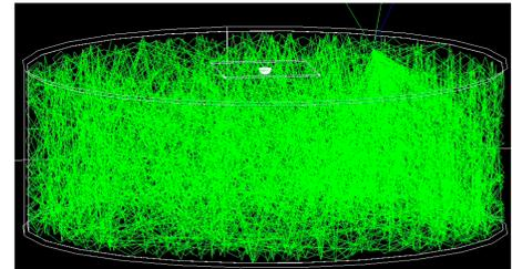
Figure 2 – An example simulation output in Geant4 using a muon to show the Cherenkov photons trajectories inside the WCD tank.
