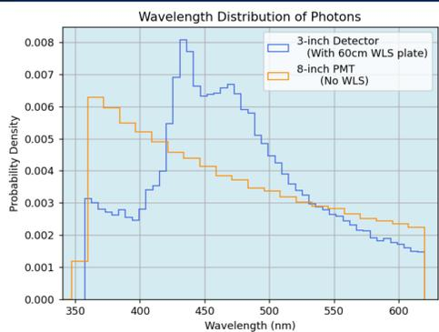
Figure 4 – Wavelength distribution for a 3-inch PMT with WLS plates and an 8-inch PMT, showing the region of shifted emission in the WLS plate.
