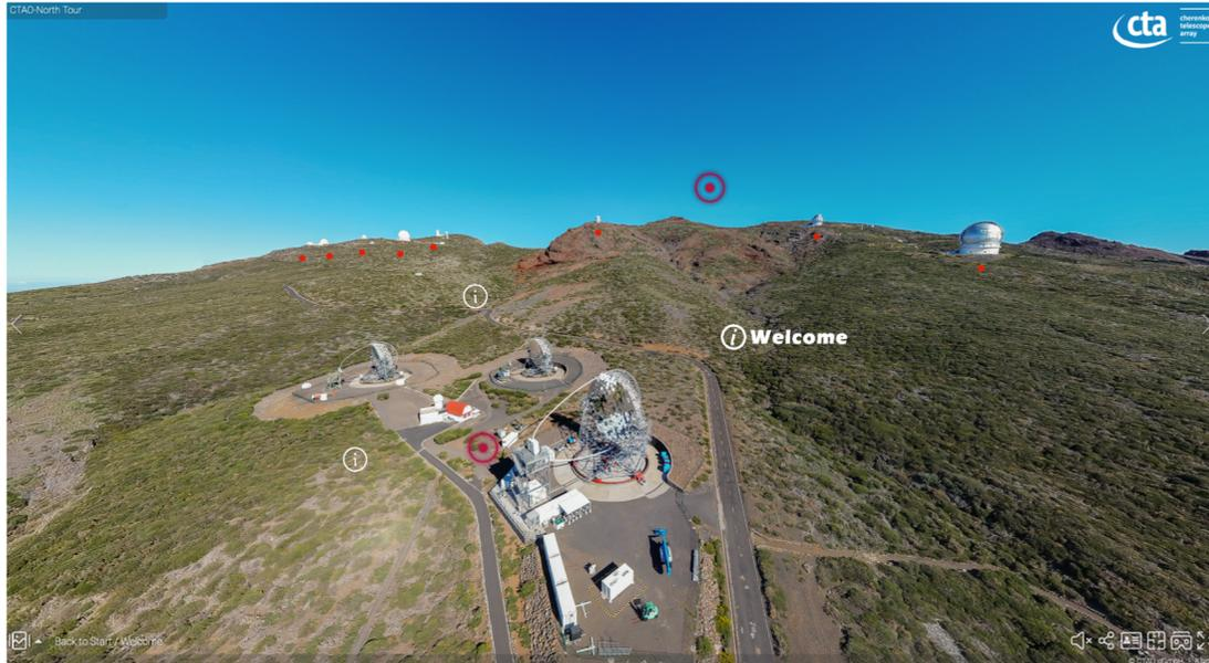
MAGIC-LST1 proximity allows joint observations for better angular & energy resolution, and better sensitivity (*Soft. and Hard. trigger*)
