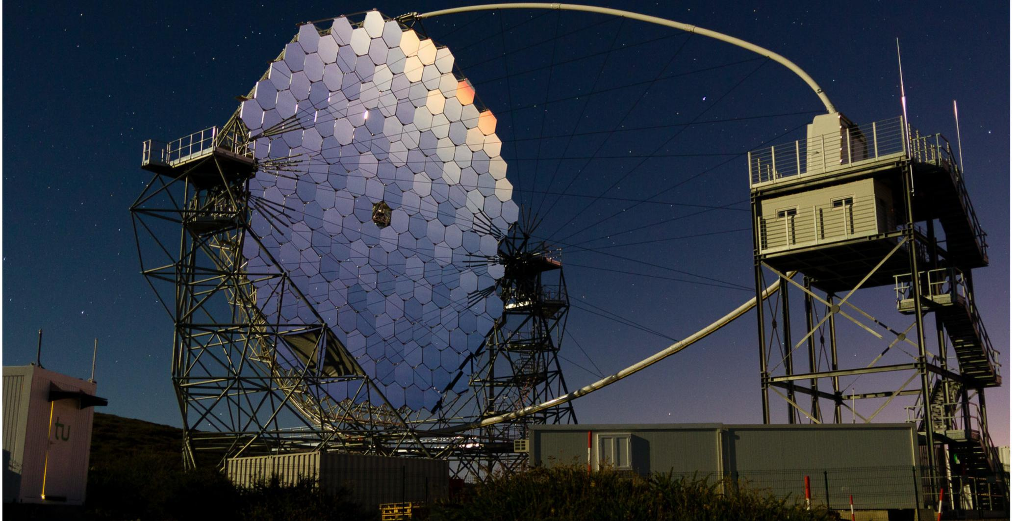
**The Large Size Telescope (LST) has a 23meter diameter mirror, that is about twice bigger than a MAGIC telescope (17 meter diam.), and the array will consist of 4 telescopes (instead of 2)**
