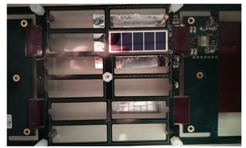
An HERMES prototype board with 10 channels, set up for testing for the SISCO project. The scintillator crystals will be attached after the first tests are concluded.
