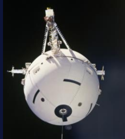
Tethered Satellite System, TSS-1, TSS-1R (space plasma physics)
