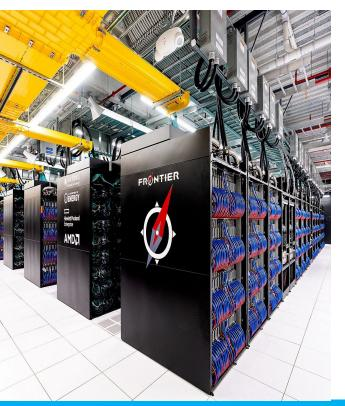
Hewlett Packard Enterprise **Frontier**, or OLCF-5, is the world's **first** and fastest **exascale supercomputer**, hosted at the Oak Ridge Leadership Computing Facility (OLCF) in Tennessee, United State.
