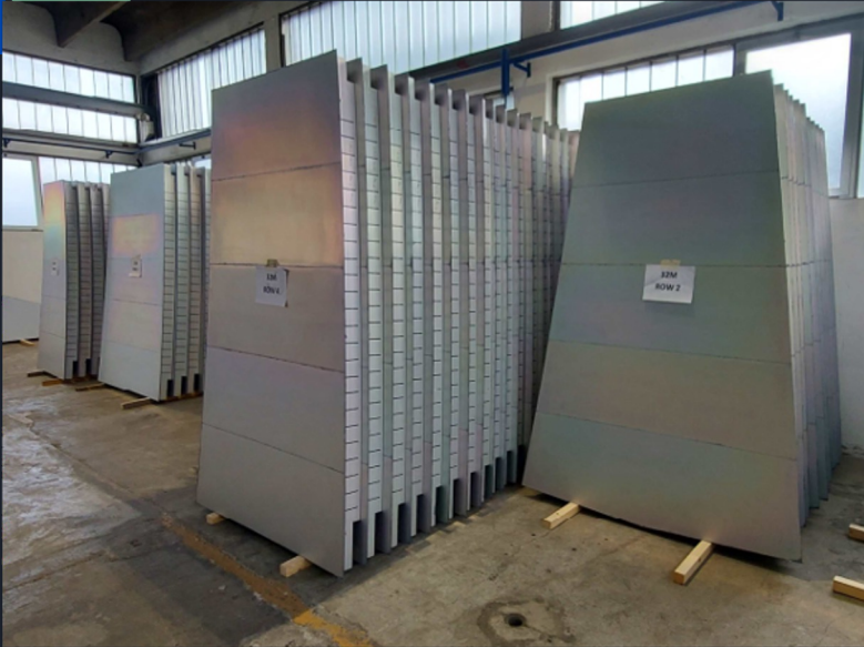
New 244 Aluminum panels forming the primary mirror of the 32m Medicina radio telescope. Manufacturing rms accuracy: \leq 65 micron Delivered.
