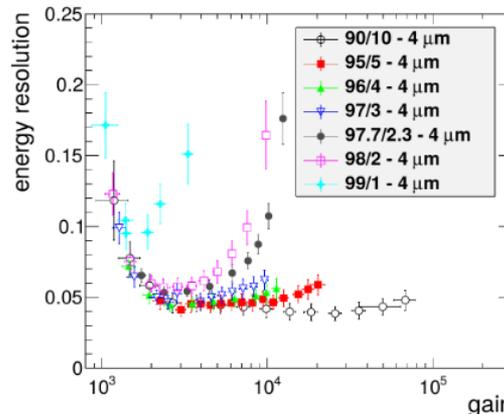
An energy resolution down to 10 % can be reached with GridPIX technologies at 6 keV
