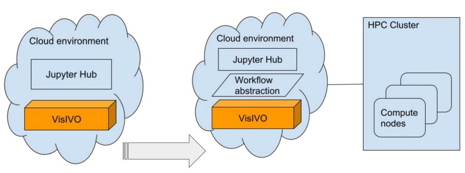
Evolution of the current Cloud deployment prototype (left diagram) toward allowing workflow abstractions and integrating HPC clusters to better exploit the parallelization of VisIVO modules.
