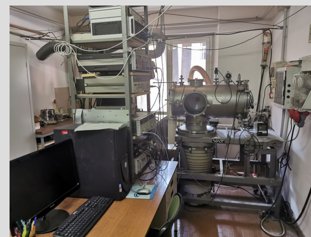
Molecular Beam Fourier Transform Microwave Spectrometer Range 6-18 GHz Resolution 0.01 MHz
