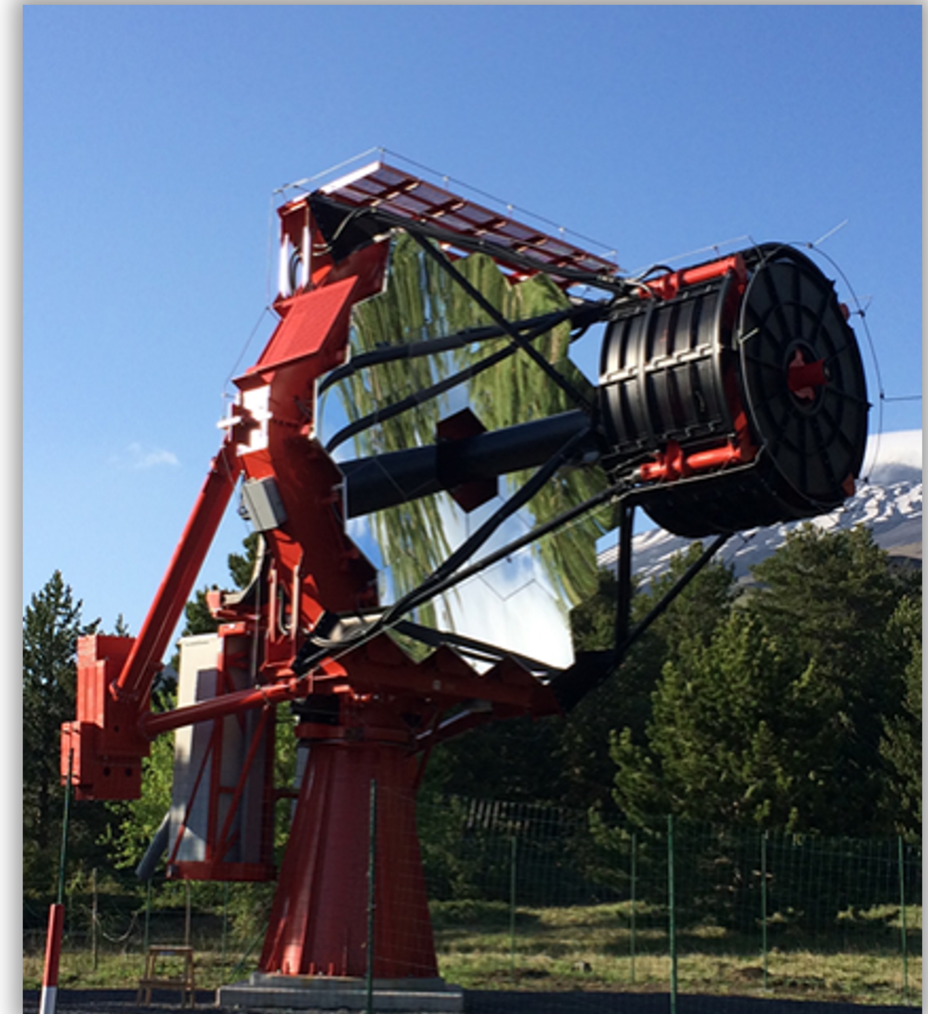
ASTRI Horn telescope at installed and operational on Mount Etna volcano (Sicily, Italy). First detection of a gamma-ray source (Crab Nebula) above 5 sigma with a dual-mirror, Schwarzschild-Couder Cherenkov telescope (Lombardi et al., 2020)
