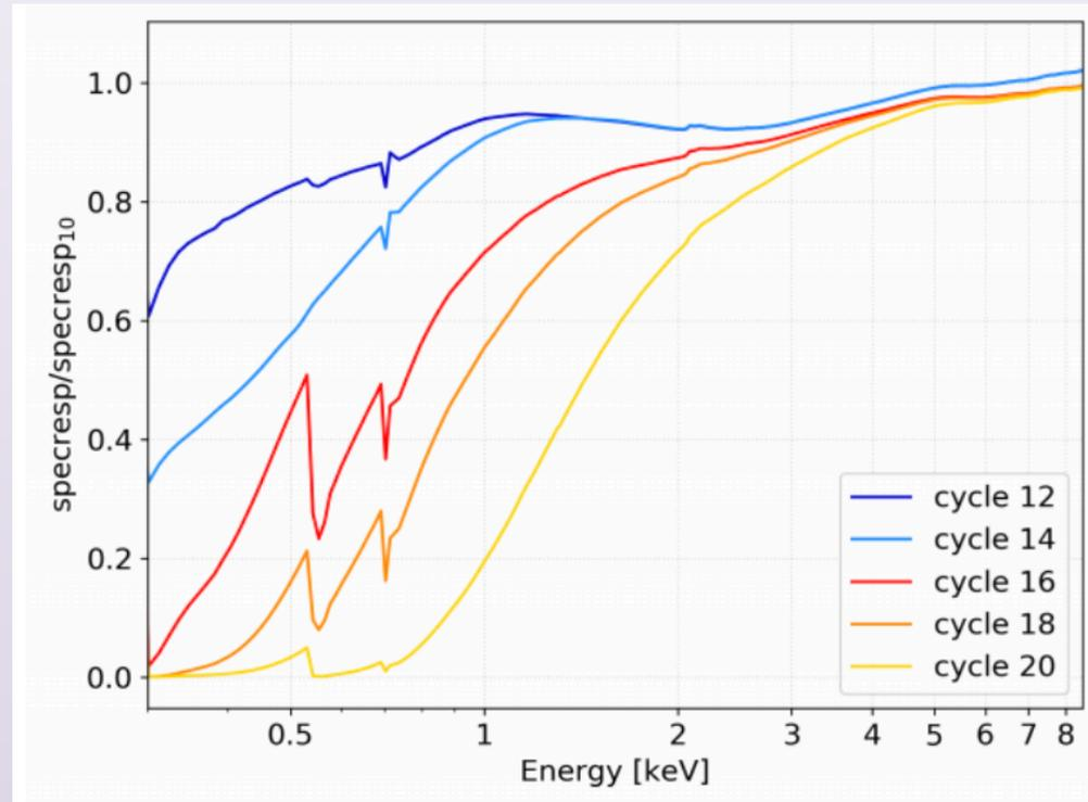
**Figure 15.** ACIS-I effective area degradation through years. We show the ARF ratios between cycles 12 (blue), 14 (light blue), 16 (red), 18 (orange), 20 (yellow) and the cycle 10.
