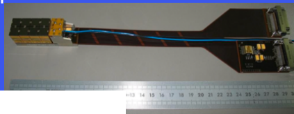
A set of Caliste modules. A version of them has been launched on Solar-Orbiter(TRL-9)
