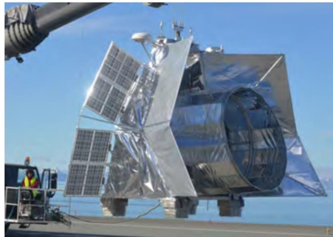
Figure 8: Two left panels: Schematic diagram of the OLIMPO instrument. From right to left: a two-mirror Ritchey-Chretien telescope feeding a cryogenic receiver with reimaging optics and four arrays at frequencies between 145 and 460 GHz. Right: The OLIMPO payload on the launch pad in Svalbard, Norway, in 2018.
