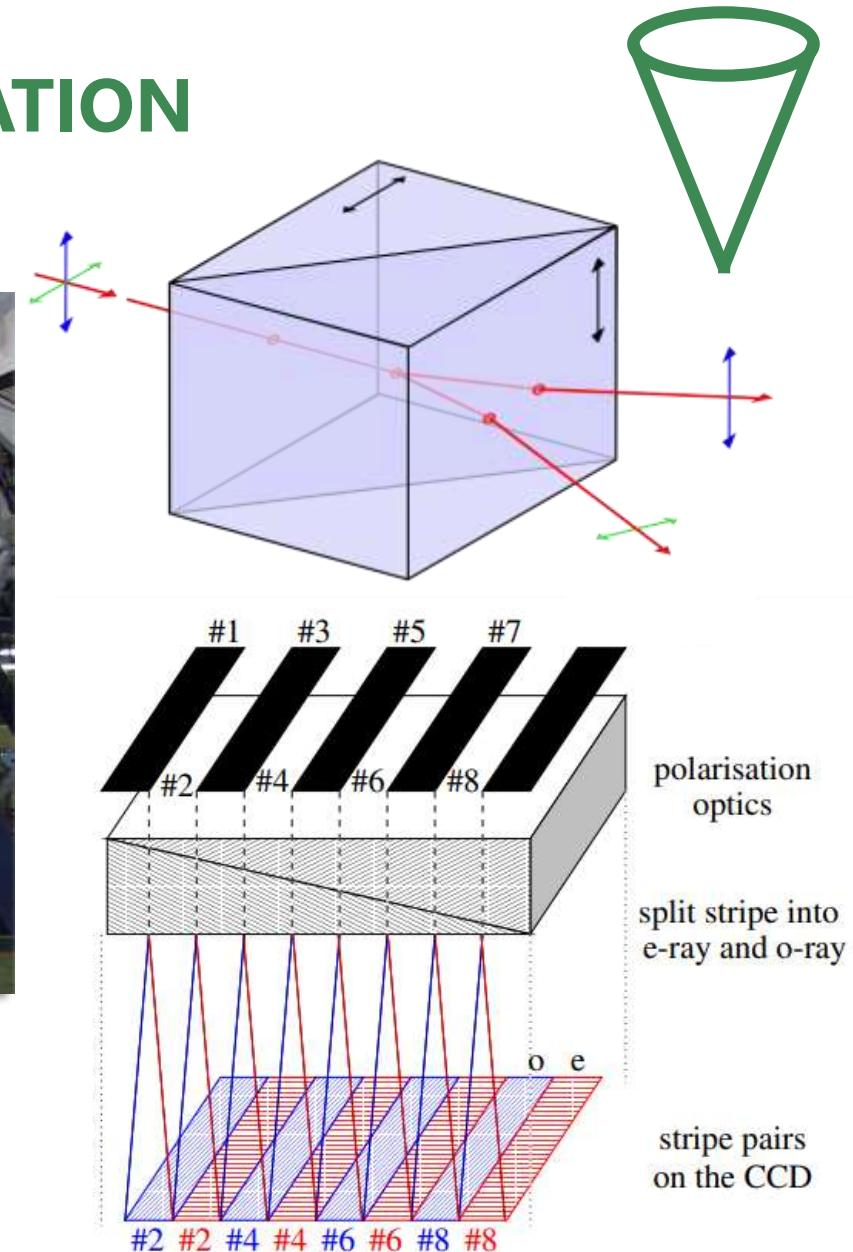
$$\frac{Q}{I} = \frac{1}{2} \left[ \left( \frac{f_o - f_e}{f_o + f_e} \right)_{0^\circ} - \left( \frac{f_o - f_e}{f_o + f_e} \right)_{45^\circ} \right]$$
