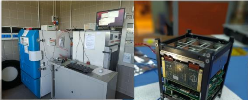
CC testing ( -30^{\circ} , +70^{\circ} , \sim 1 \text{ m}^3 )
