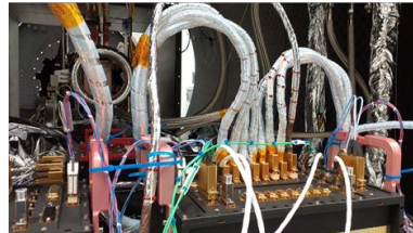
NISP warm electronics: 2 x Data Processing Units (top), Instrument Control Unit (bottom)
