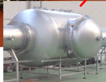
Thermostated telescope chamber: 200 cm diam., 350 cm long. Equipped with Alt-Azimuth mount.
