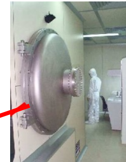
The detector test chamber opens inside an ISO 6 cleanroom.
