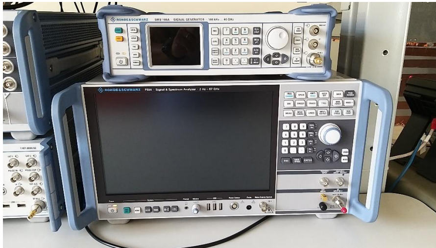
FSW – Signal & Spectrum Analyzer 2 Hz – 67 GHz
