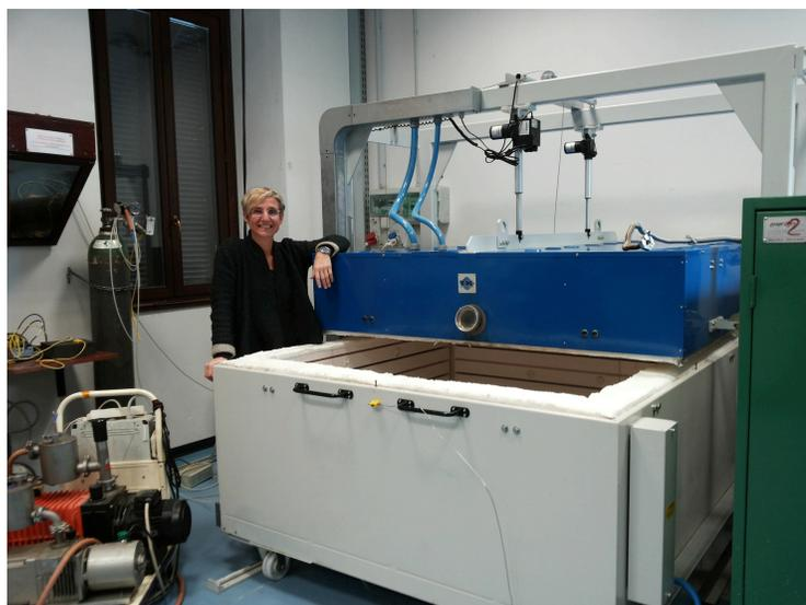
The oven for hot forming of thin glass foils
