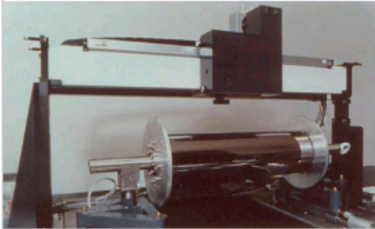
**Dimetior Vbe ESDI:** Fizeau interferometer with vibration compensation and high-rate acquisition. Resolution  $< \lambda/8000$ , accuracy  $< \lambda/100$ .
