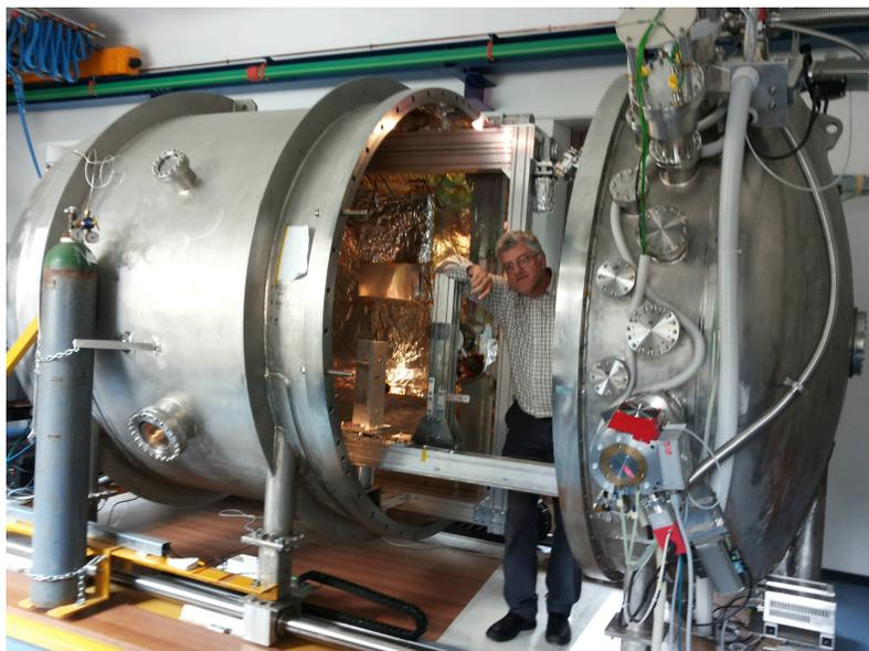
The Ion Beam Figuring vacuum facility
