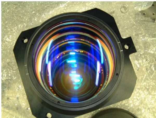
Ø130mm very fast (f/0.88) objective for LBT-NIRVANA wavefront sensor
