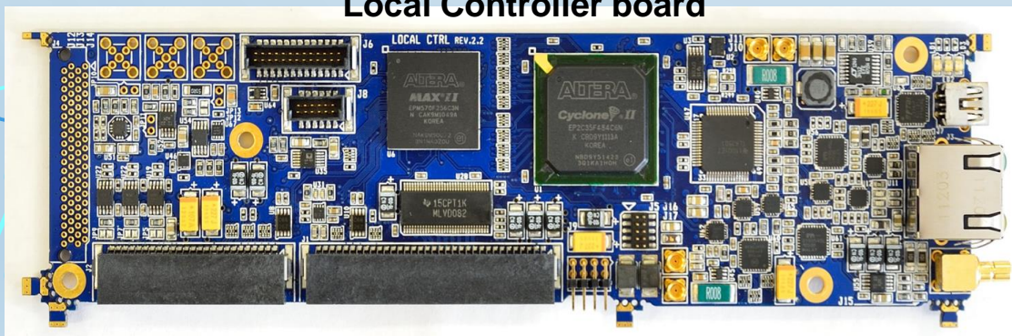
Local Controller board
