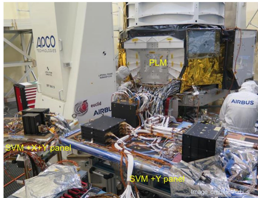
E-PLM ELECTRICAL SETUP FOR ART #1 (AMBIENT REFERENCE TESTS):
