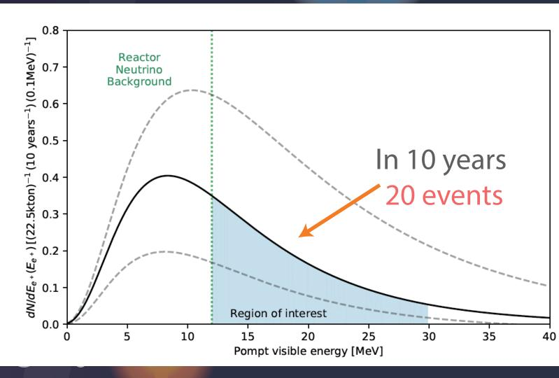
In SK-Gd, the DSNB signal is dominated by the reactor neutrino background at energies below 12 MeV [3]. In the region of interest (12–30 MeV), the fiducial model predicts 20 events in 10 years for a fiducial volume of 22.5 kt and a delayed neutron detection efficiency of 67 %.
