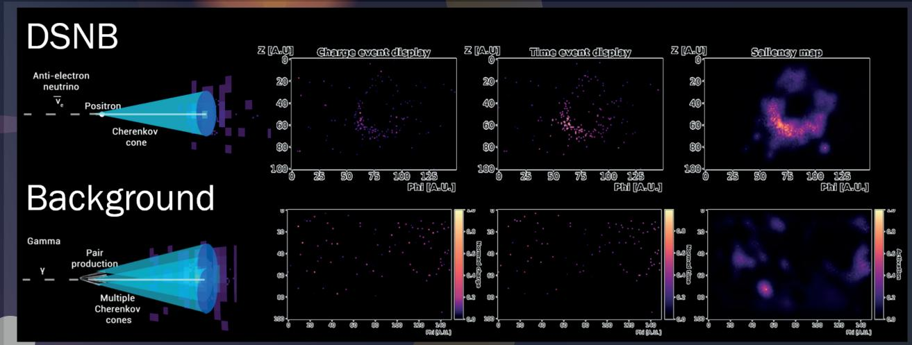
The DSNB and NCQE data, which was generated in MC simulations, is converted into a pixelized image we call a "hit map", conceptually close to a conventional event display. The collected charge (photo electrons, p.e.) per PMT and first photon arrival time are translated into two hit maps in which each PMT is assorted to a specific pixel. Pixels in both hit maps are normalized to a range from 0 to 1. 15.000 images
