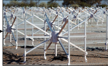
EDA2 - 256 MWA dipoles with modified LNA for 50-350 MHz
