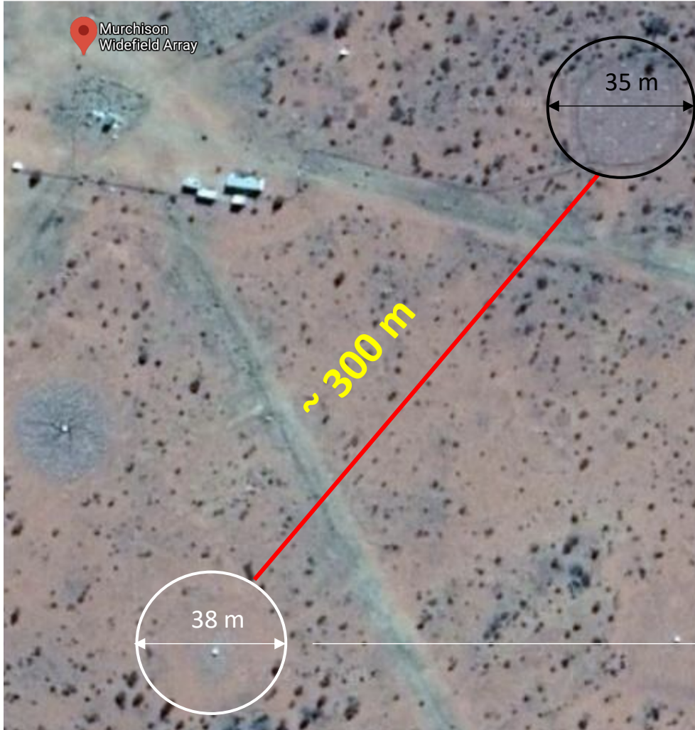
AAVS2 – 256 SKALA 4.1 log periodic antennas SKALA 4.1 passed the critical design review
