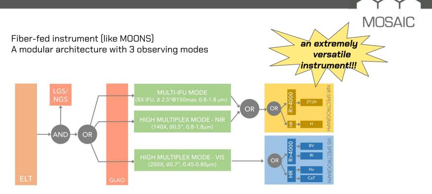
MOSAIC combines the advantages of a highly-multiplexed (HMM) instrument targeting numerous unresolved sources, both in the VIS and in the NIR, with one having a more modest multiplex but that can resolve faint sources spatially (multi-IFU- NIR only ).
