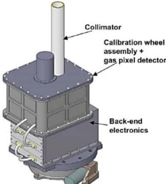
Figure E-4: Detector Assembly with Back-End Electronics on Turntable
