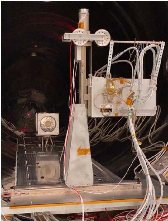
SLTF Telescope Calibration configuration
