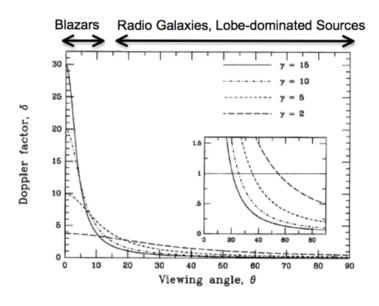
Doppler factor  $\delta = [\Gamma (1 - \beta \cos\theta)]^{-1}$  $\Gamma = (1 - \beta^2)^{-1/2}$  bulk Lorentz factor,  $\theta$  viewing angle
