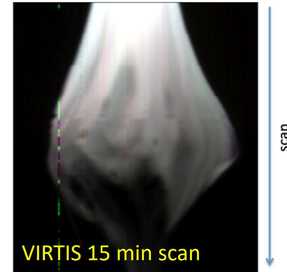
*Rosetta's flyby of asteroid 21 Lutetia on July 10th 2010 (minimum distance 3162 km, fly-by velocity 15 km/s) evidences the limitations of pushbroom spectrometers like VIRTIS.*
