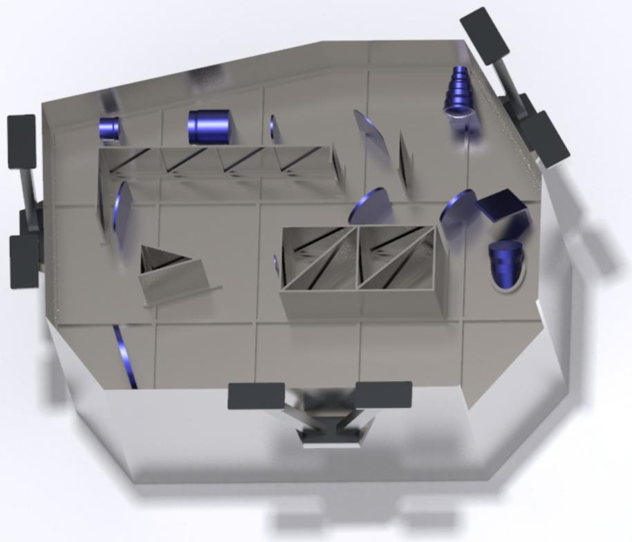
Telescope and Imager optical bench (bottom side)
