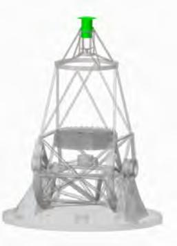
**Lot 3:** Preliminary design of the **adaptive secondary mirror (M2)** of the European Solar Telescope
