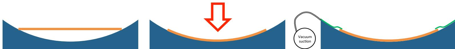
Precise positioning and ribs gluing by means of IMA (Integration MMachine) @ INAF-OAB:
