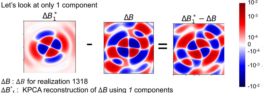
$\Delta B_{1}^{*} - \Delta B$ : the difference between the KPCA reconstruction using 1 components and  $\Delta B$
