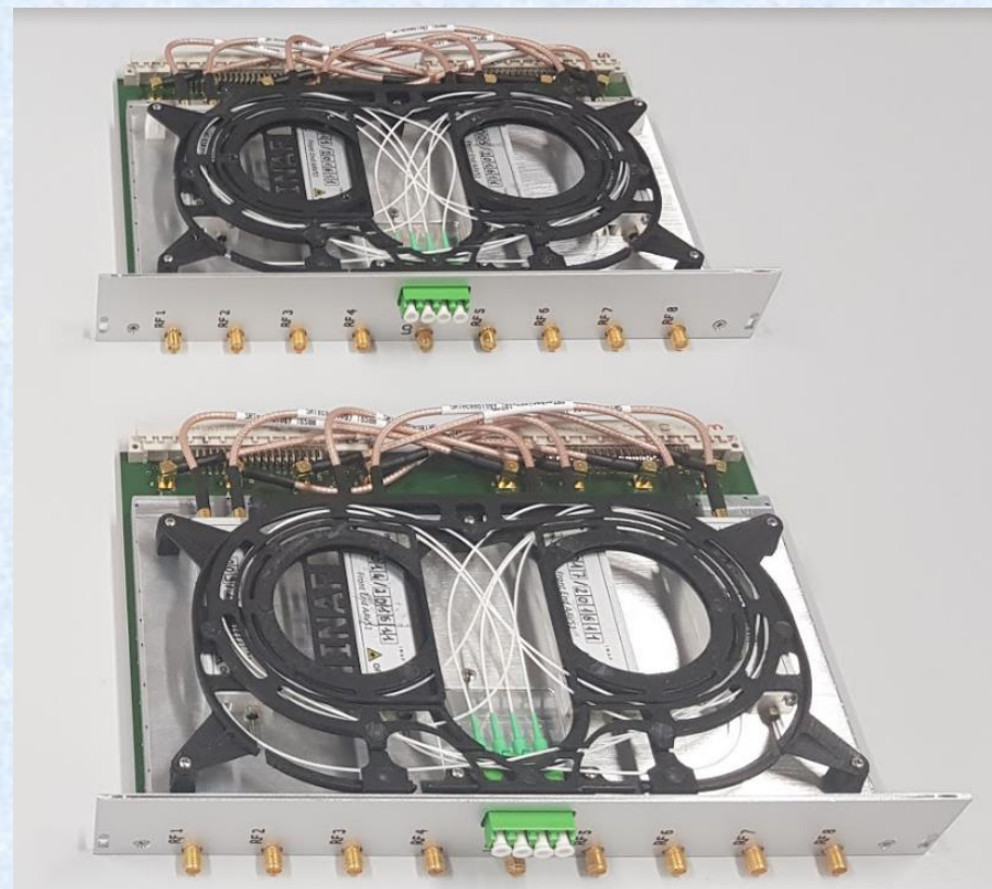
Two eight-channel modules assembled with IF over fiber (IFoF) optical transmitters:
