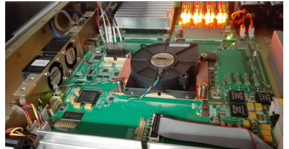
Square Kilometer Array Reconfigurable Application Board (SKARAB)
