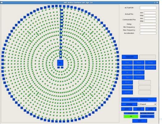
• The AS subsys set each of the 1116 actuators to its elongation for commanded elevation
